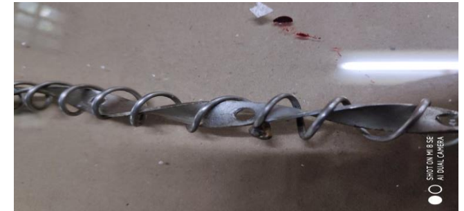
Fig. 3: Photographic view of coiled perforated twisted tape insert
